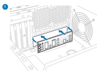
1. Install the ASUS Q-Shield to the chassis rear I/O panel.
