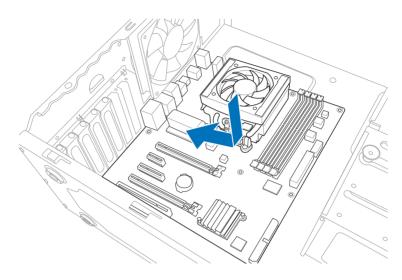
3. Place nine screws into the holes indicated by circles to secure the motherboard to the chassis.
