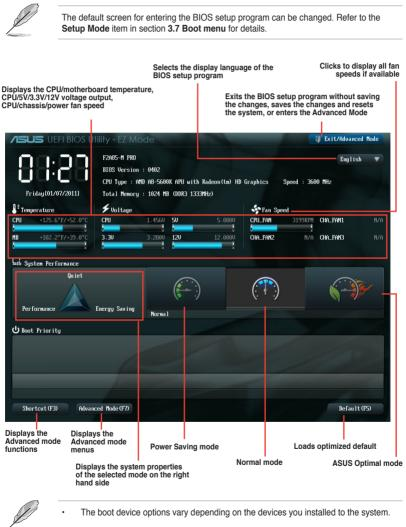
The Boot Menu(F8) button is available only when the boot device is installed to the system.
